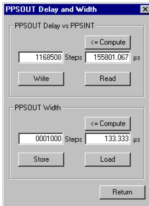
Figure 13 - PPS OUT Delay & Width Settings
