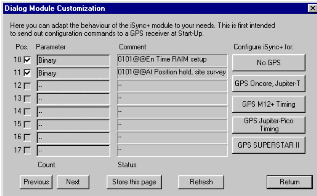
**Figure 16 - GPS Configuration Settings at Startup**
