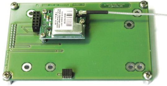
Figure 7 – Installing Navman Jupiter Pico T on the GPS Interface Board
