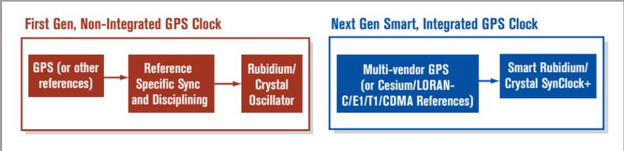
Figure 1. First vs. Next Generation GPS/Multi-Reference Clock designs
