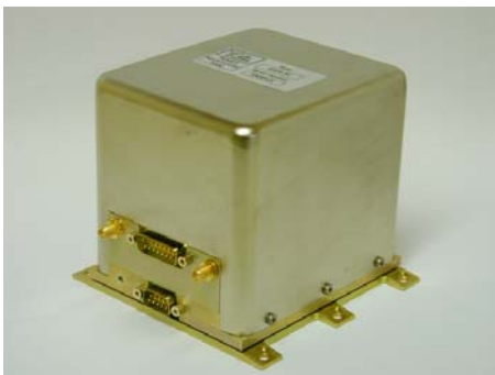
Figure 1. Picture of the updated RAFS1 once closed including the thermally regulated base plate
