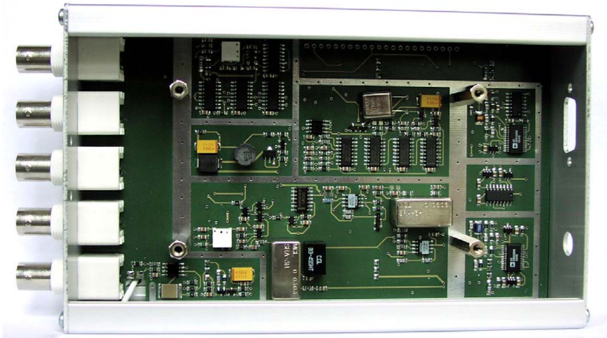
Fig. 3 : PicoTime open box showing RF circuitry
